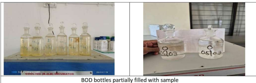
BOD bottles partially filled with sample
